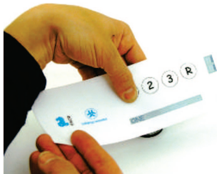
Figure 33. System-on-a-sheet demonstrator developed by Linköping University and the Acreo Institute (Sweden). PEDOT/PSS-based electrochemical transistors, displays, logic, and batteries are combined into a stand-alone label demonstrator. Adapted with permission from ref 425. Copyright 2007 Nature Publishing Group.
