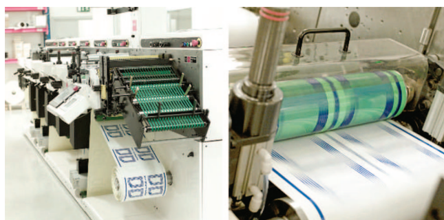
Figure 34. Nilpeter rotolabel FA3300/5 printing press at the Acreo Institute where flexoprinting, rotary printing, screen printing, and offset printing can be combined. Flexoprinting (where the ink is transferred from a cylinder) is commonly used in packaging technology and patterning with speeds exceeding 100 \text{ m min}^{-1} . Paper and plastic-based active-matrix displays could ultimately be manufactured in a roll-to-roll process via this type of high-speed printer. Adapted with permission from ref 425. Copyright 2007 Nature Publishing Group.
